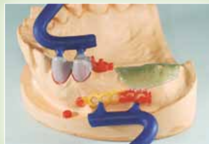
Before spruing and investing, be sure to remove the positioning ring from the OT CAP sphere.
